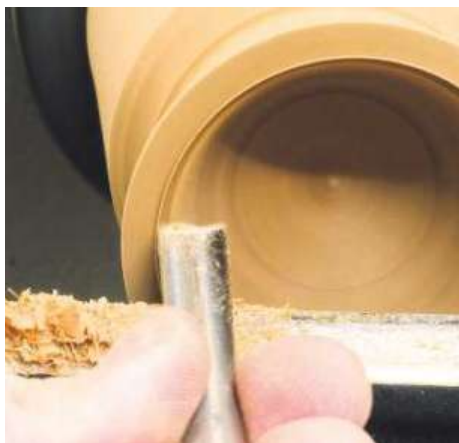
▲ Pic.10 Once you have achieved the basic shape you will need to cut a recess for the lid to fit into. It will need to be a nice fit but the size can be adjusted on the lid part
